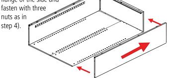
6. Attach the sill (Ref. No. 8) to the sides. Place nuts loosely on each of the studs and slide the ends of the sill into the slots on both sides of the unit. Then, securely tighten the nuts.
