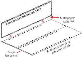
4. Attach the top (Ref. No. 5) to the unit by sliding the outer flange over the back of the unit and the side flange on the top over the side panel. The
