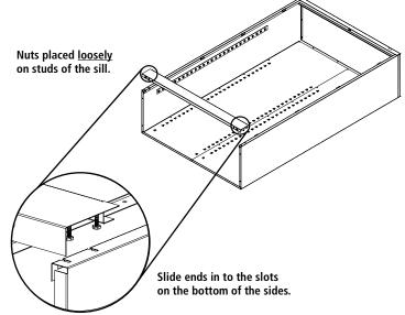
7. Place the rear flange of one of the shelves (Ref. No. 4) into the four bottom lances of the back. The front of the shelf will rest on the sill.
